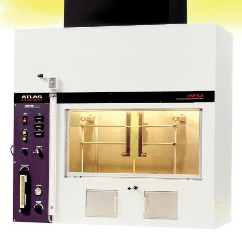
Atlas' HVFAA Horizontal Vertical Flame Chamber accurately determines the flammability of cabin compartment materials and electric wire. The chamber is designed to perform Bunsen burner tests in accordance with FAA's *Aircraft Material Fire Test Handbook* DOT/ FAA/AR-00/12, chapters 1.0 - 4.0 (FAR 25.853, 25.855, 25.1359).
