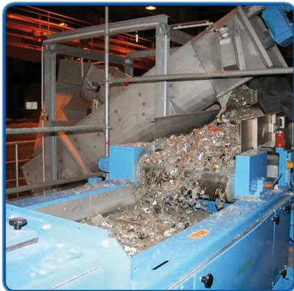
Depending on the application the eddy current separator type 0428 is available in dust proof variation. It is possible to build the machine with peak roller at the separation edge and automatic rotating brush for belt cleaning.
