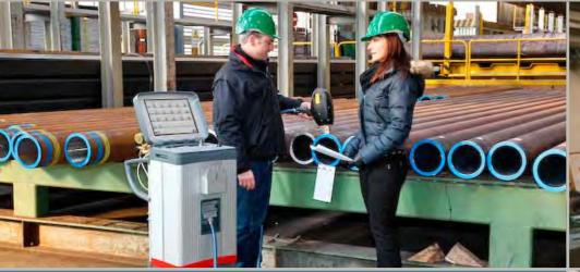
**Mobile Metal Analyzer** Highest Analytical Performance and Maximum Sample Throughput
