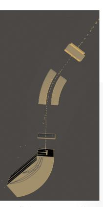
Simultaneous measurement of the entire spectrum is enabled by the combination of double focusing sector field mass spectrometer and a novel planar detector.
