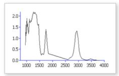
A typical IR spectrum from FluidScan
