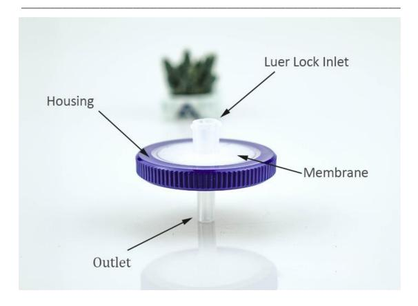
It is essential that the right selection of syringe filters is chosen to ensure reliable testing results and best purifying performance. **Membrane diameters, materials, pore size,** and **housing** all affect the right choice. Here we'll walk through the important factors to help you make the right choice compatible.
