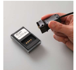
● Check the probe by probe checker.
